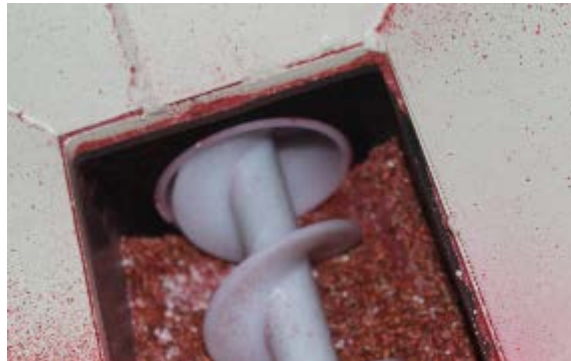
No impact on metering auger
